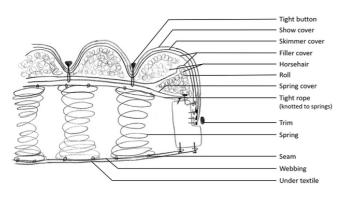
Figure 1: Diagram of the cross-section of the sprung upholstered seat based on documentation. Diagram by Margot Dubost, copyright Nationalmuseum, Sweden.
