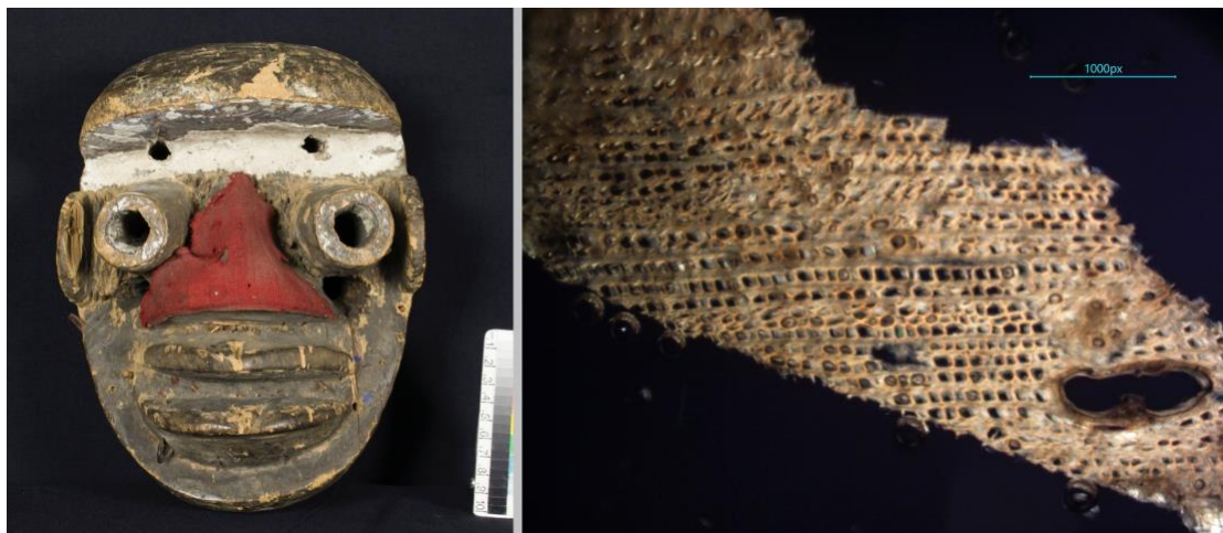
Figure 3: (Left): Mask. Unknown Artist. Dan style, Liberia. c. early 20 th century. Wood, pigment and cloth. Gift of the Wellcome Trust, X65.4783; Fowler Museum at UCLA. (Right): Wood section (taken from X65.4783) under cross-polarized light microscopy. The resin canal (ovular feature, bottom right in section) and wood tissue composed of mostly tracheids informs this mask to be made from a softwood species of tree.
