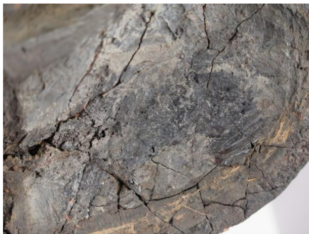
Figure 4: Detail of the embrittlement of the black resin (Courtesy of A. De Paepe, Collection of Royal Museum for Central Africa, Tervuren©).
