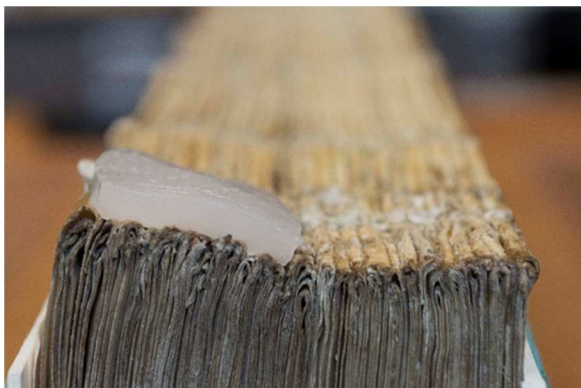
Fig. 2: The ability of HAGG to conform to the uneven book spine was instrumental to the success of the gel. © Image courtesy of the Walters Art Museum, Baltimore.
