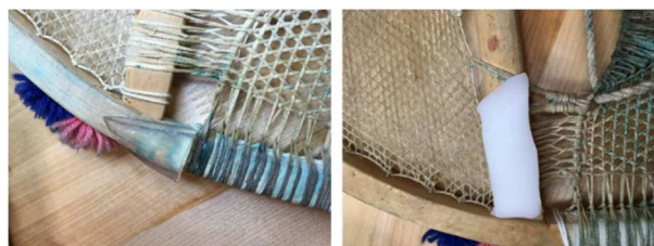
Fig. 3: 2% LAGG gellan gum test on snowshoe (left), 2% HAGG gellan gum test on snowshoe (right).
