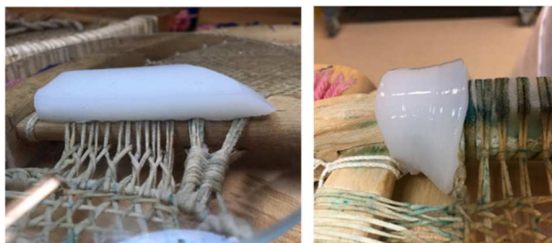
Fig. 5: 2 cm thick piece of 2.5% HAGG gel conforming to snowshoe shape (left), 1cm thick piece of 2.5% HAGG gel conforming to bend in snowshoe (right).
