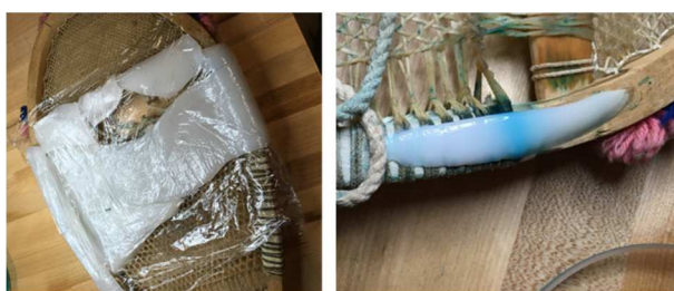
Fig. 6: General application of the HAGG gel covered with plastic (left), localized application of the HAGG gel after 6 hrs (right).
