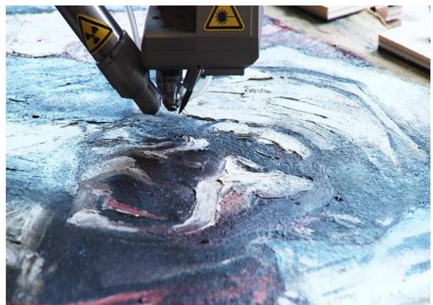
The paint layer has been analysed using micro X-ray fluorescence analysis (micro-XRF).
