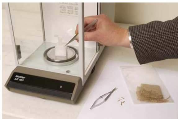
Figure 2. Weighing a 0.0010 g fibre sample. By taring the balance and placing the fibre on the foam jig, it is quick and easy to weigh samples to 0.0010 g. All fibre is then transferred into the snap cap micro centrifuge tube.
