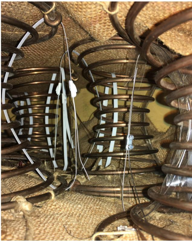
Figure 3: Compressing the springs from the inside with polyester-coated stainless steel cable ties (left) and the first metal system (right). Photo by Margot Dubost, copyright Nationalmuseum, Sweden.
