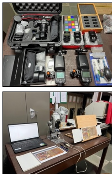
Figure 2. Top: multispectral imaging (or technical photography) kit components from the MCH India mobile heritage lab.
