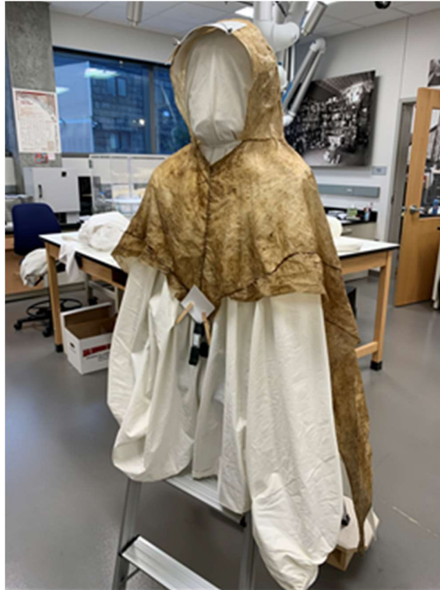
Figure 5. Treatment of a hood and cape made of whale intestine, showing clips and blotter paper to reshape humidified areas. (TD.2023-7-7).
