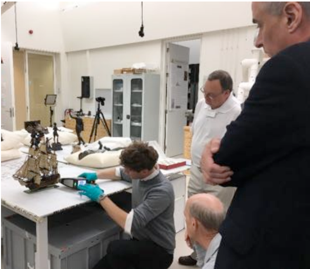
Arie Pappot demonstrates portable XRF (Bruker) using a ship model from the collection of the Rijksmuseum.
