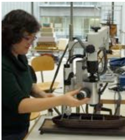
Davina Kuh Jakobi sets up the equipment to examine the tool marks of a ship model from the collection of the Rijksmuseum. On the right, Jolanda van Iperen demonstrates digital microscopy using the Hirox RH-2000 in the furniture and ship model conservation atelier at the Rijksmuseum.
