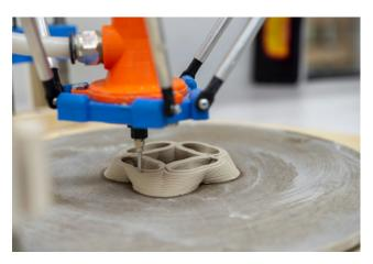
Ceramic object being 3D printed through material extrusion. ©Rochester Institute of Technology, Grace Walker.
