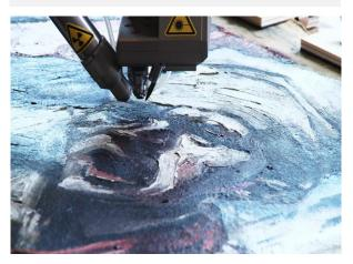
The paint layer has been analysed using micro X-ray fluorescence analysis (micro-XRF).
