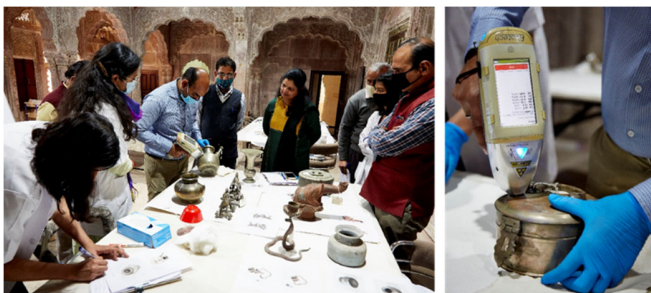
The XRF technician shows how the measurements are made using the HH-XRF instrument, Hand-held XRF Analysis
