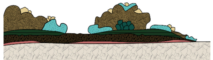
Top: the cross-section under bright field. Bottom: an interpreted stratigraphy: Probable but unidentified copper bromide (pink), silver chloride (black), green copper corrosion products, copper chlorides (light green) and sediments (brown).
