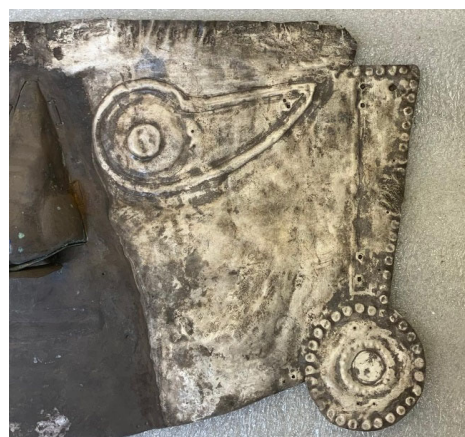
Top: The mask covered with a layer of sodium dithionite in Laponite that is turning brown after 30 minutes, indicating a reduction of the silver chloride. Bottom: Some darker areas remaining after EDTA and sodium dithionite treatment.
