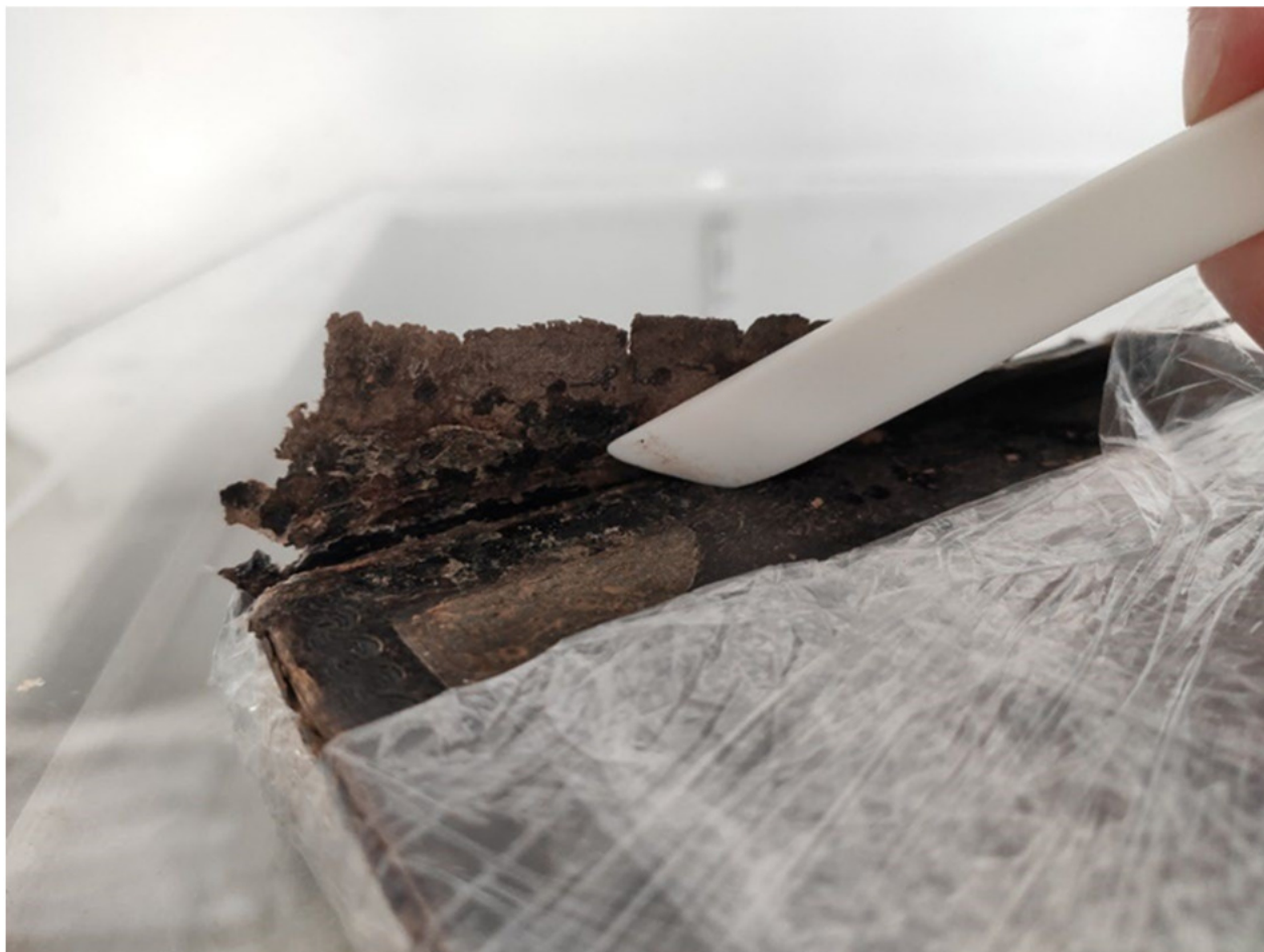
Figure 1: After 30 min. inside the solvent chamber, the repair leather was easily removable using a spatula. Before being placed inside the chamber, the inner book and most of the binding were covered in transparent foil to shield them from the solvent fumes.
