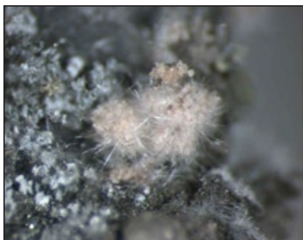
Fig.3 Efflorescence analysed by XRD - römerite \text{Fe}^{2+}\text{Fe}^{3+}_2(\text{SO}_4)_4 \cdot 14\text{H}_2\text{O} , forms at higher temperatures and humidity
