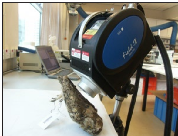
Fig 1 XRF set up for the analysis of an owl specimen
