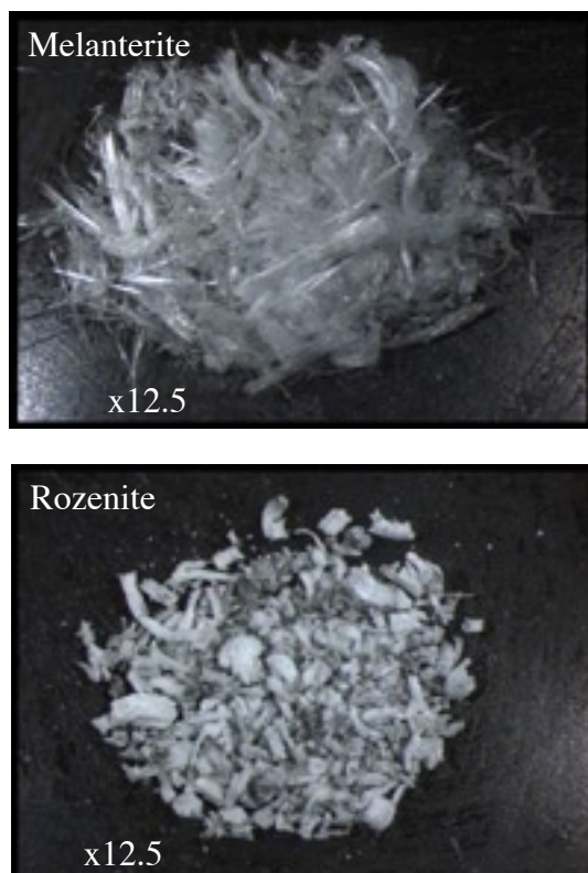
Fig.6 Post project decay showed the melanterite \text{FeSO}_4 \cdot 7\text{H}_2\text{O} when removed from its high humidity environment, dehydrated to rozenite \text{FeSO}_4 \cdot 4\text{H}_2\text{O}
