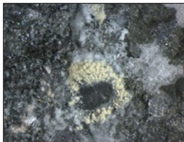
Fig.5 Efflorescence analysed by XRD - magnesiocopiapate \text{MgFe}^{3+}_4(\text{SO}_4)_6(\text{OH})_2 \cdot 2\text{OH}_2\text{O} formed in higher humidity with an interaction with the host rock
