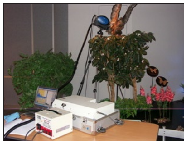
Fig 4 XRF set up for the analysis of eagle in the Science Museum
