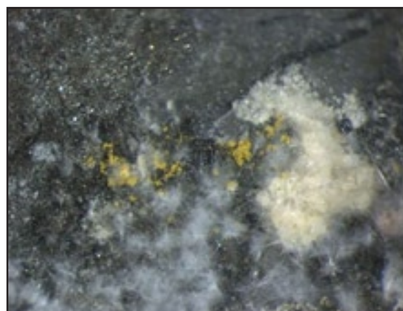
Fig.4 Efflorescence analysed by XRD - akaganeite \text{Fe}^{3+}\text{O}(\text{OH}) , natural rust
