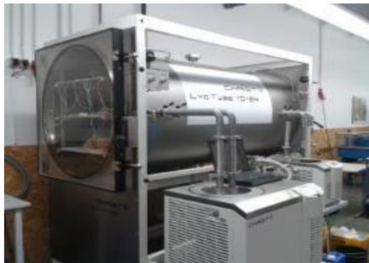
Fig 4: Vacuum freeze drying unit in Cologne
