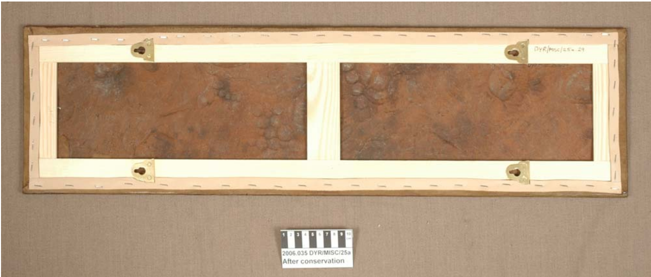
Fig. 4. The leather attached to the frames with Monel staples.
